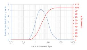
Typical particle size distribution for product 0-20  $\mu$ m. Measurements by laser diffraction (Malvern mastersizer 2000).
