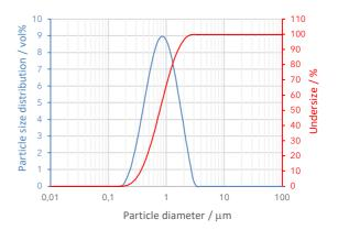
Typical particle size distribution. Measurements by laser diffraction (Malvern Panalytical Mastersizer 2000).
