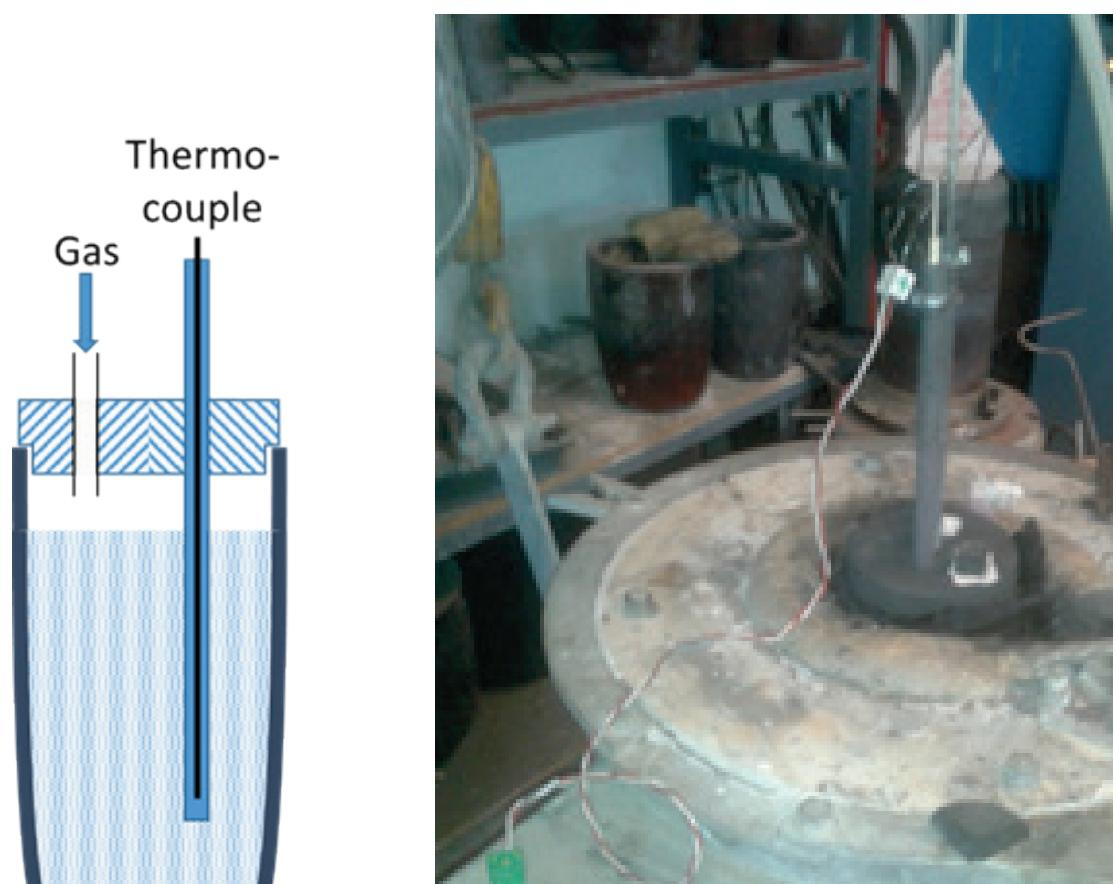
An inductively heated furnace with graphite crucible and lid is used for melting and refining, and a Crystalox DS250 furnace is used for directional solidification. The chamber above the charge is continuously flushed with argon to minimize oxidation.
