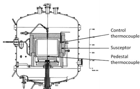
The Crystalox DS250 furnace at SINTEF was used for the tests with directional solidification. The furnace produce 12 kg ingots.
