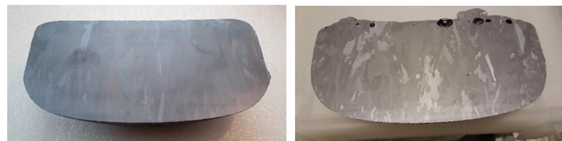
The 10 % ingot showed normal grain structure whereas the 100 % ingot had lost the planar crystallization front due to too high impurity level.
