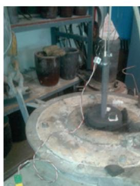
An inductively heated furnace with graphite crucible and lid is used for melting and refining, and a Crystalox DS250 furnace is used for directional solidification. The chamber above the charge is continuously flushed with argon to minimize oxidation.
