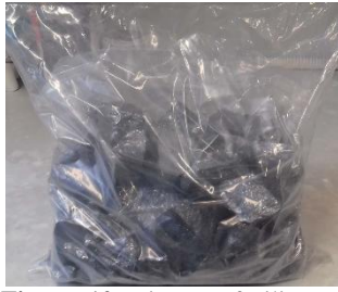
Figure 10: Picture of silicon chunks from melted and solidified material with its origin in Si-kerf.
