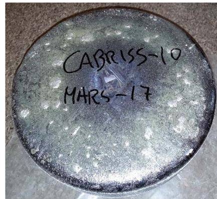
Figure 5: Photo of the ingot with 10 % refined material and 90 % poly-Si.
