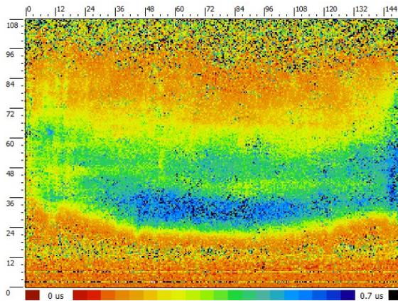
Figure 10: Lifetime mapping of the side of the 10 % ingot.
