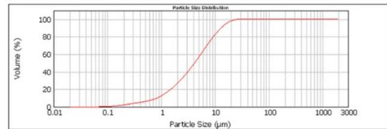
Figure 1: Size distribution of the silicon powder from ReSiTec.
