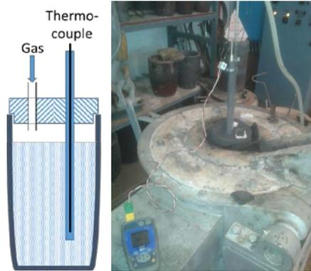
Figure 4: Schematic of the melting and separation setup on the left hand side and a photo of the experimental setup at the right. The inner diameter of the crucible is 150 mm and about 300 mm inner height.
