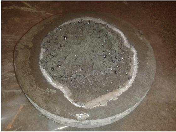
Figure 2: Photo of the first crystallisation test of the provided powder from ReSiTec.
